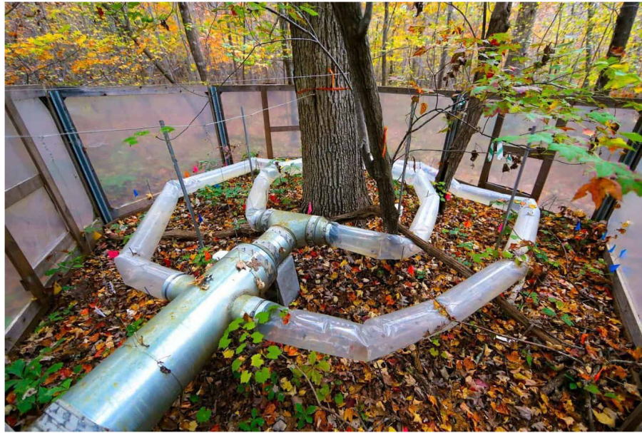
Fig. 1. Warming chamber at Duke Forest, North Carolina, USA. The chambers were 5 m in diameter and warmed by heated air blown through vents surrounding a central white oak ( Quercus alba ) (photo: James Waters).
